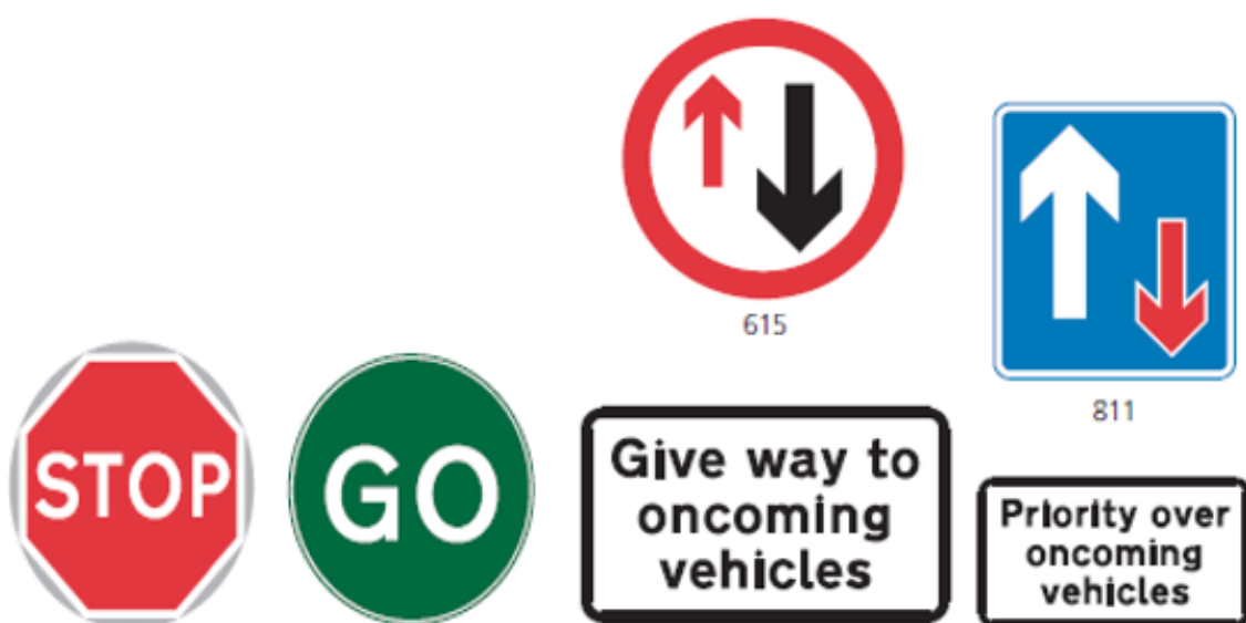
Figure 1.5: Manually operated stop/go signs and priority signs
